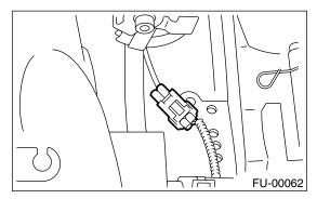
4) Remove the knock sensor from the cylinder block.
