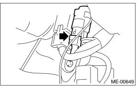
15) Connect the battery ground cable to battery.
