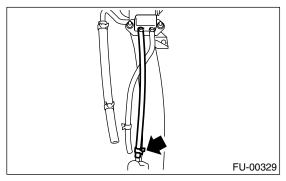
2) Remove the bolt which installs the joint pipe on fuel filler pipe.
