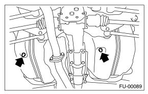
10) Tighten the fuel drain plug and then install the front right side tank cover.
