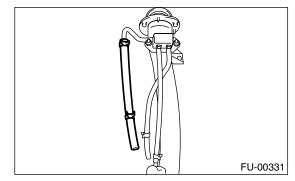
4) Remove the shut valve from the fuel filler pipe. <Ref. to EC(STi)-17, REMOVAL, Shut Valve.>
