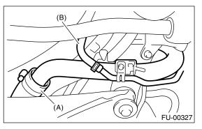
17) Remove the fuel filler pipe to the underside of vehicle.
