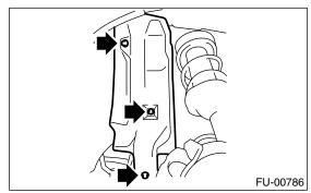
12) Separate the evaporation hoses from the clip of fuel filler pipe.
