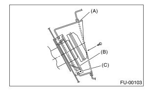
4) Install the evaporation pipes.
