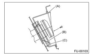
3) Align the holes in fuel filler pipe neck and set the cup (B), and tighten the screws.
