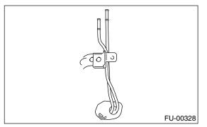
5) Connect the evaporation hose to pipes.
