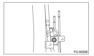
15) Loosen the clamp, and disconnect the fuel filler hose (A) from fuel filler pipe.
