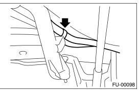
13) Disconnect the evaporation hoses from the pipes.
