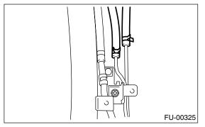
14) Remove the bolts which hold fuel filler pipe bracket on the body.
