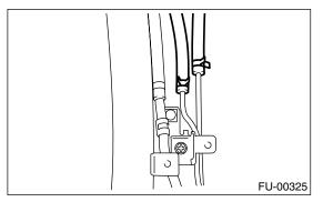
6) Insert the fuel filler hose (A) approx. 35 to 40 mm (1.38 to 1.57 in) over the lower end of fuel filler pipe, and then tighten the clamp.
