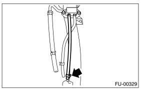
4) Install the evaporation pipe to the fuel filler pipe.
