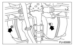
11) Remove the fuel filler pipe protector.
