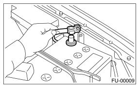
5) Remove the screws holding packing.
