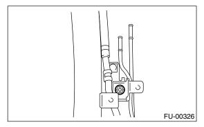
9) Tighten the bolts which hold evaporation hoses onto the clip of fuel filler pipe.
