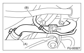
7) Insert the air vent hose approx. 25 to 30 mm (0.98 to 1.18 in) into the lower end of air vent pipe, and then hold the clip.
