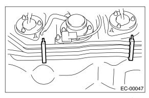
5) Remove the bolt and nut which hold the fuel tank pressure sensor onto the bracket.
