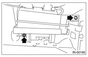
5) Remove the hose between body and water tank, then remove the water tank.
