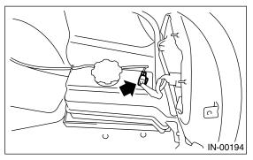
4) Remove the two water tank installation bolts.
