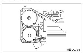
(2) Set the arrow mark on camshaft sprocket to position shown in the figure, and then measure the #2 cylinder intake valve and #4 cylinder exhaust valve clearances.
