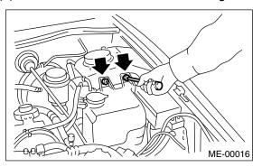
(5) Move the washer tank upward.
