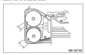
(3) Set the arrow mark on camshaft sprocket to position shown in the figure, and then measure the #1 cylinder exhaust valve and #4 cylinder intake valve clearances.
