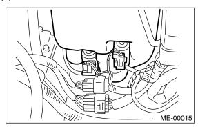
(4) Remove the washer tank mounting bolts.
