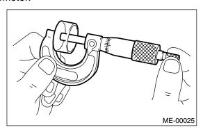
5) Select a valve lifter of suitable thickness using measured valve clearance and valve lifter thickness, by referring to the following table.
