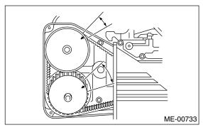
12) Measure the #1 cylinder intake valve and #3 cylinder exhaust valve clearance by using thickness gauge (A).
