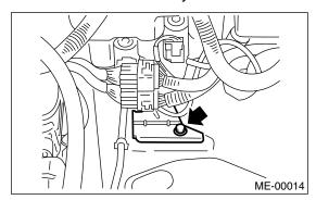
(3) Disconnect the washer motor connectors.
