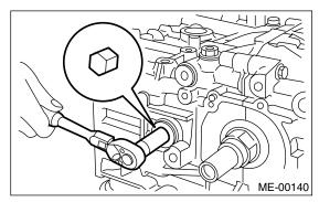
24) Rotate the crankshaft to bring #1 and #2 pistons to bottom dead center position, and then remove the piston circlip through service hole of #1 and #2 cylinders.
