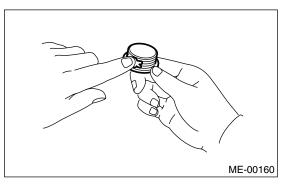
(5) Install the service hole plug and gasket.
