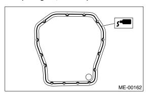
27) Apply fluid packing to the matching surfaces, and then install the oil separator cover.
