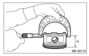
5) Calculate the clearance between cylinder and piston.
