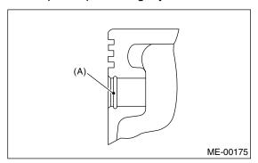
5) Check the piston pin circlip for distortion, cracks and wear.
