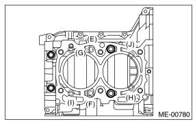
11) Tighten the 8 mm and 6 mm cylinder block connecting bolts in alphabetical sequence shown in the figure.
