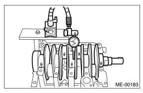
3) Inspect the crank journal and crank pin for wear. If they are not within the specifications, replace the bearing with a suitable (undersize) one, and then replace or recondition the crankshaft as necessary. When grinding the crank journal or crank pin, finish them to specified dimensions according to the undersize bearing to be used.
