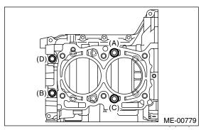
6) Tighten the 10 mm cylinder block connecting bolts in alphabetical sequence shown in the figure. (RH side)
