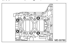
9) Further tighten the LH side bolts (A — D) by  $90^{\circ}$  in alphabetical sequence.
