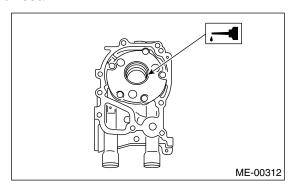
(4) Install the oil pump on cylinder block. Be careful not to damage the oil seal during installation.
