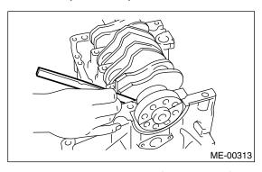
5) Inspect individual crankshaft bearings for signs of flaking, seizure, melting, and wear.
