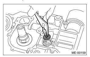
(4) Apply fluid packing around the service hole plug.
