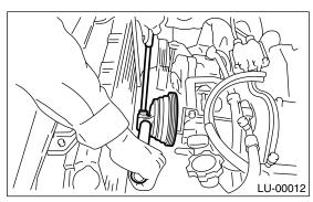
11) Remove the water pump. <Ref. to CO(H4DOTC)-19, REMOVAL, Water Pump.> 12) Remove the timing belt guide.
