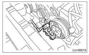
15) Remove the oil pump using the flat tip screw-driver.
