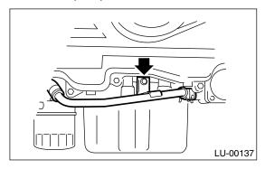
5) Remove the water pipe and hoses between oil cooler and water pump.
