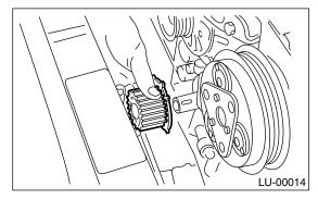
14) Remove the bolts which install the oil pump onto cylinder block.
