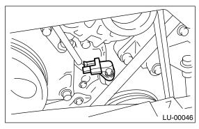
8) Remove the V-belts. <Ref. to ME(STi)-41, REMOVAL, V-belt.> 9) Remove the rear side V-belt tensioner.
