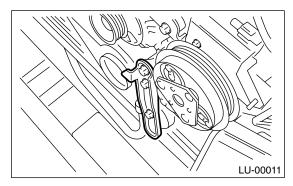
10) Remove the crankshaft pulley by using ST. <Ref. to ME(STi)-44, REMOVAL, Crankshaft Pulley.>
