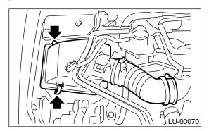
14) Connect the connector to mass air flow sensor.
