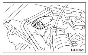
5) Remove the air intake boot and air cleaner upper cover.
