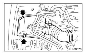
6) Remove the intercooler. <Ref. to IN(H4DOTC)-10, REMOVAL, Intercooler.>
