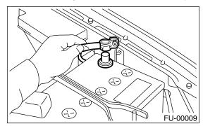
4) Disconnect the connector from mass air flow sensor.
