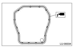
4) Tighten the bolts which install the oil pan onto engine block.
