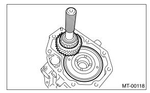
2) Remove the bearing outer race from the extension case.
