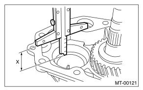
6) Calculate the space "t" using the following equation: t = X - W + 0.2 to 0.3 mm (0.008 to 0.012 in) 7) Select the nearest washer in the following table:
