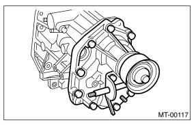
17) Install the shifter arm to transfer case.
