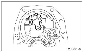
2) Install the reverse check sleeve assembly to transfer case. <Ref. to 5MT-48, INSTALLATION, Reverse Check Sleeve.>
