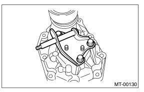
3) Remove the oil seal from extension case. <Ref. to 5MT-34, Oil Seal.>
