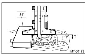
12) Calculate the space "U" using the following equation: U = S + T - 30 mm (1.18 in) [Thickness of ST]
