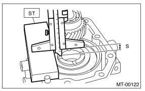
11) Measure the depth "T" between extension case and transfer drive gear.
