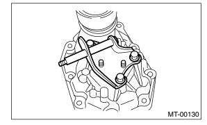
3) Install the transfer drive gear to extension case. <Ref. to 5MT-43, INSTALLATION, Transfer Drive Gear.>
