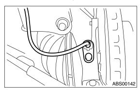
2) Install the front ABS wheel speed sensor on strut and wheel apron bracket.
