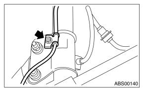
4) Remove the bolts which secure the sensor harness to body.
