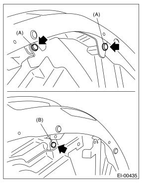
6) Remove the four clips in the center part of bumper.
