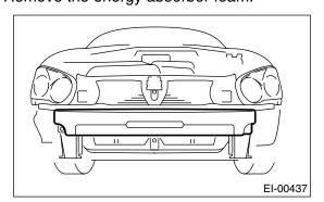
10) Loosen the bolt and nut, and then remove the bumper beam from body.
