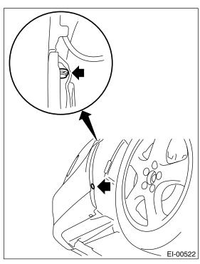
5) Remove the two clips (A), turn over the mud guard, and then remove the clip (B). (Conduct the same procedure on the right side.)
