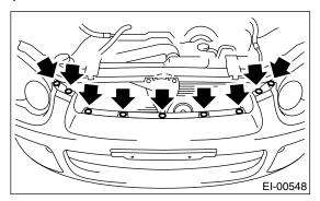
4) Turn over the mud guard, and then remove the clips (A) and (B), which secure the front bumper to fender.
