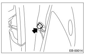
11) Remove the door-side bolts for upper and lower hinges to remove the rear door panel.
