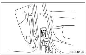
9) Put a wooden block on the jack and place the jack under the rear door. Support the rear door with jack to protect it.
