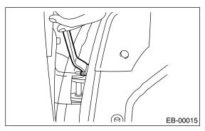
2) Loosen the screw (A), and then tap striker (B) using plastic hammer to adjust striker to align the position of rear door panel laterally at the rear end.
