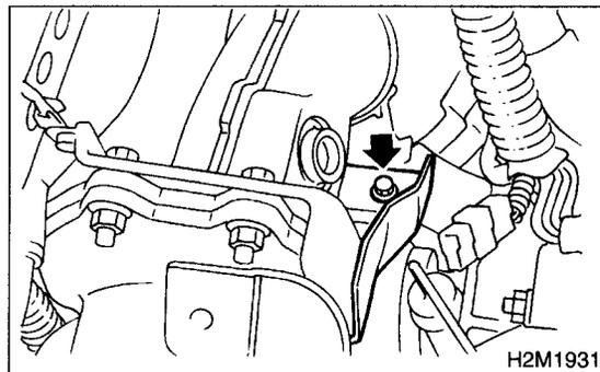
12) Place the turbocharger upper cover, and tighten the bolts which install the upper side of upper cover.
